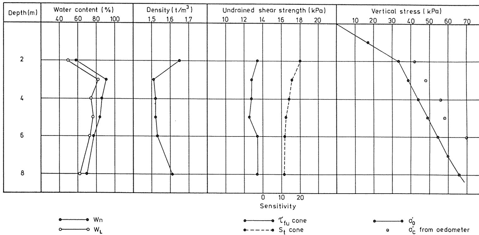
Fig. 6. Characteristics of Tornby clay.
