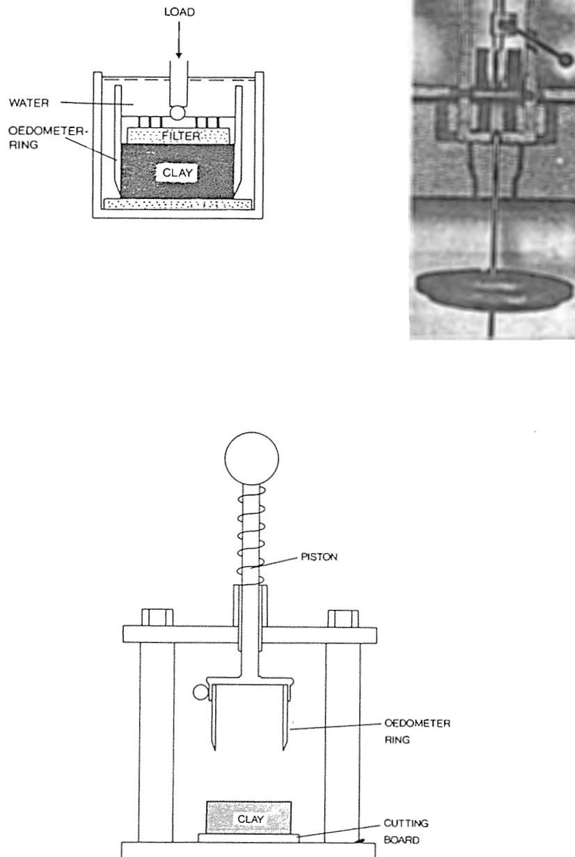
Fig. 3. Apparatus in incremental oedometer tests (a) and cutting device used for mounting clay sample (b).
