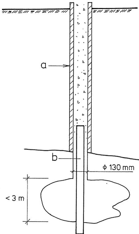
Fig. 3d Small hollow pile for small cavities,
