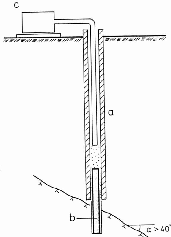
Fig. 3a Small hollow pile for the case of steep sloping bed rock ( $\alpha > 40^\circ$ )
