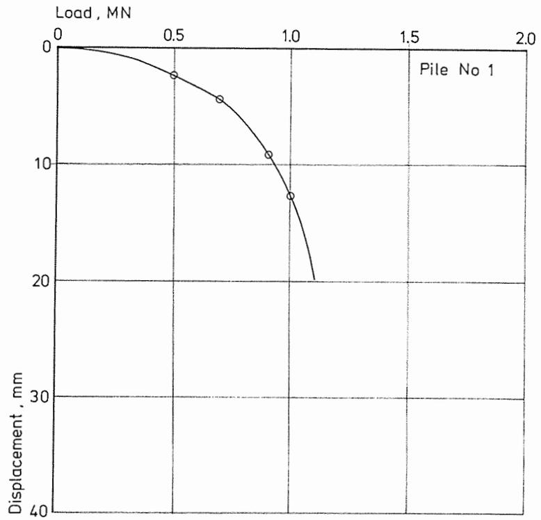
Fig. 5a Load displacement curve for pile 1.
