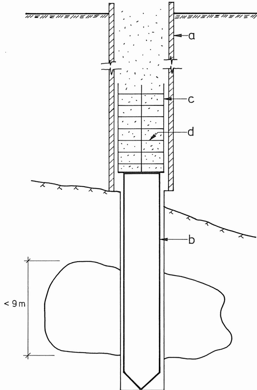
Fig. 4 Great concrete pile and steel pile
