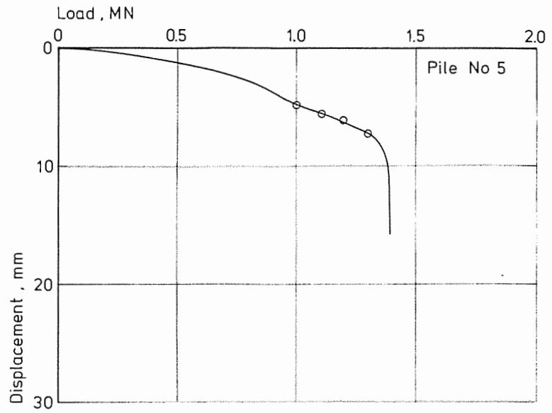
Fig. 5e Load displacement curve for pile 5.
