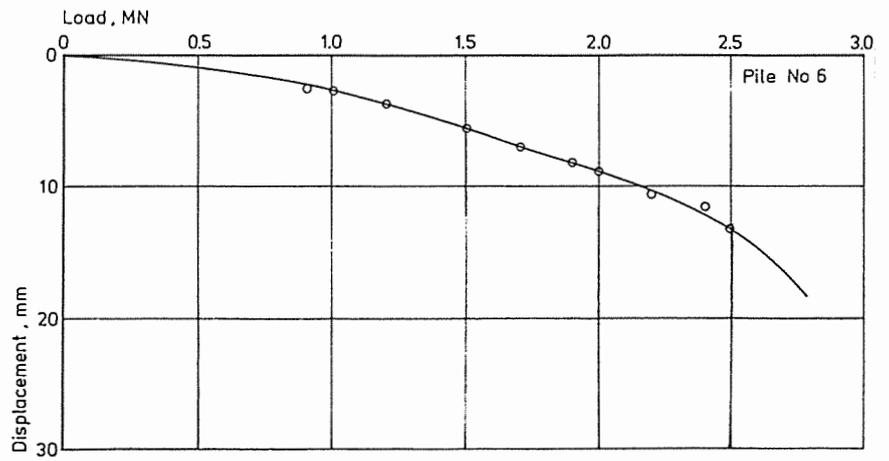
Fig. 5f Load displacement curve for pile 6.
