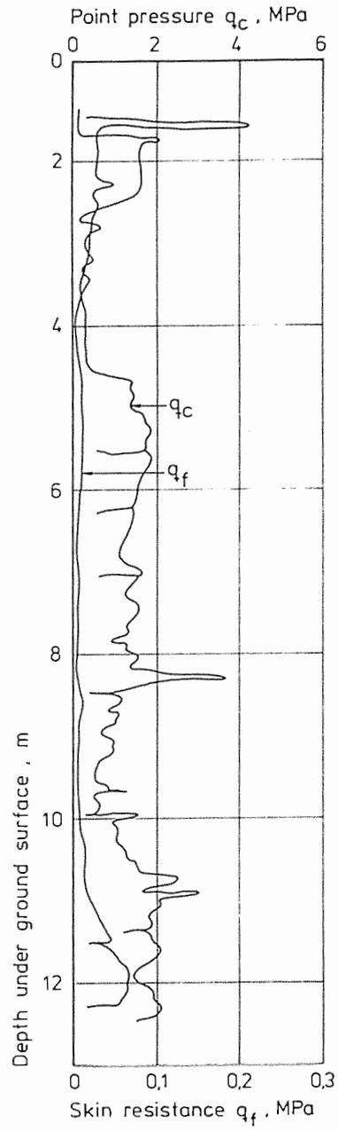
Fig. 1 Typical result of static sounding.
