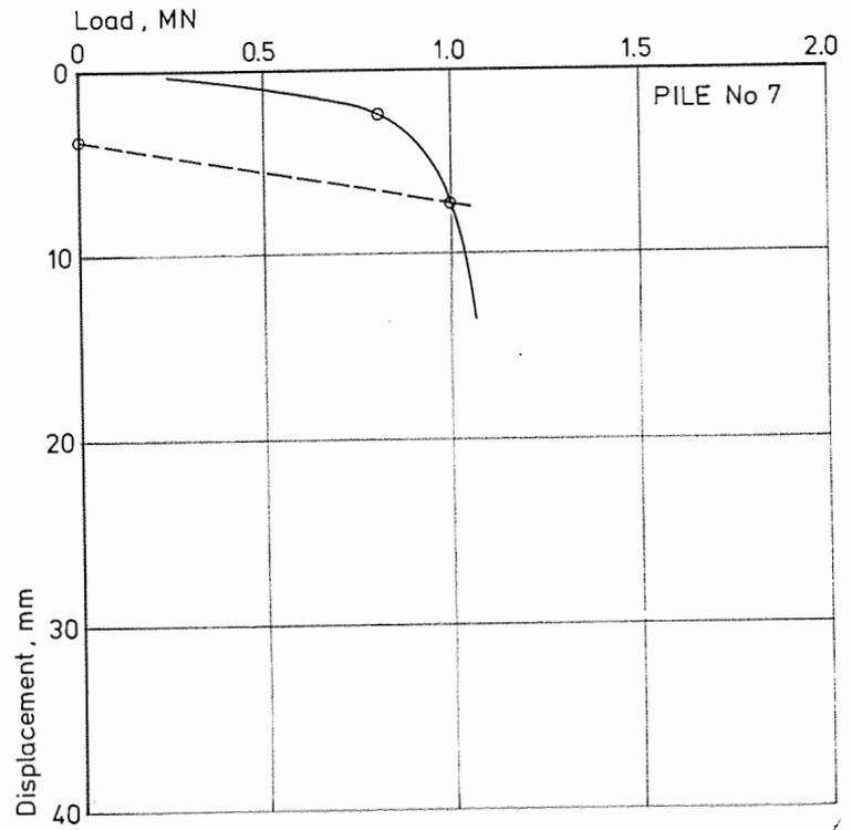
Fig. 5g Load displacement curve for pile 7.
