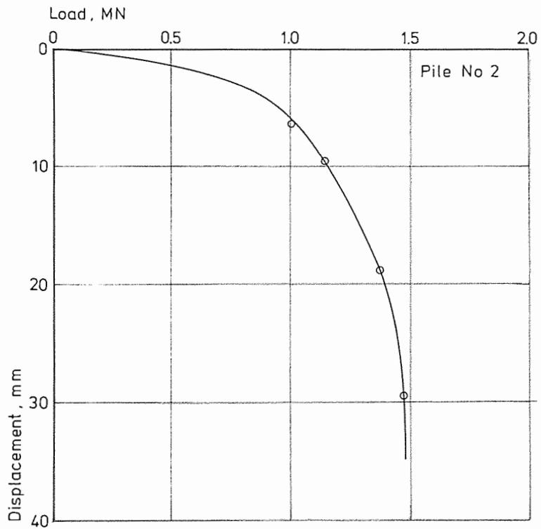
Fig. 5b Load displacement curve for pile 2.
