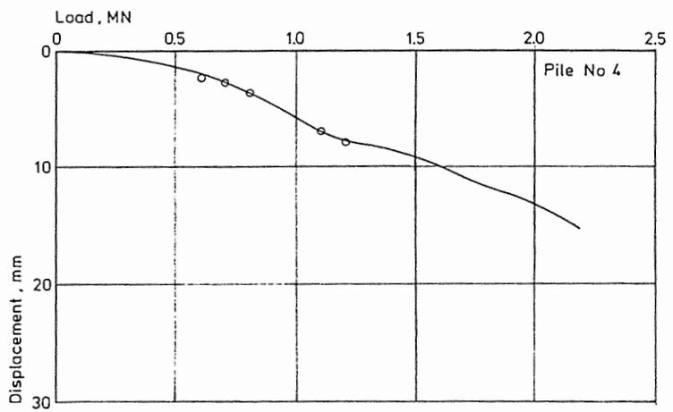
Fig. 5d Load displacement curve for pile 4.
