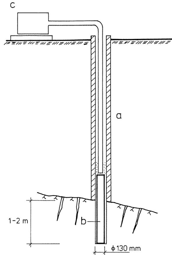
Fig. 3b Small hollow pile for the case of weathered bed rock
