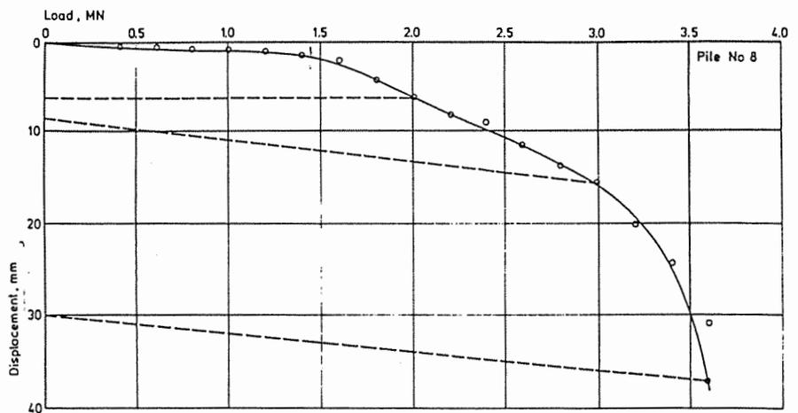
Fig. 5h Load displacement curve for pile 8.
