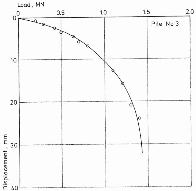
Fig. 5c Load displacement curve for pile 3.
