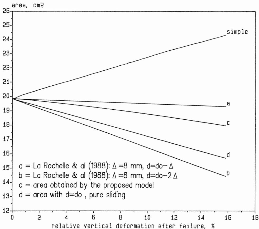
Fig. 6. Development of the vertical strain area calculated by different methods for testing silty clay soil containing 10% cement (failure strain is 1.38%).
