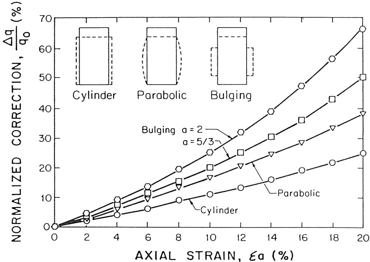
Fig. 1. Typical modes of area development for specimen submitted to triaxial testing, with relative influence on deviator stress at the constant volume compression (after [1]).
