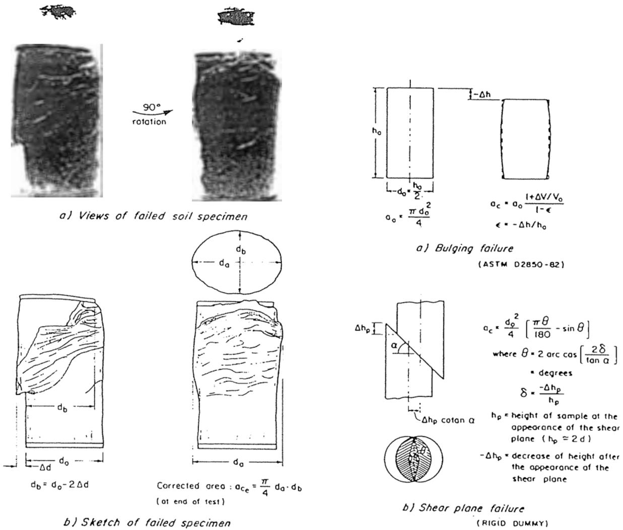
Fig. 2. Shear plane failure in a soil specimen (after [5]).
