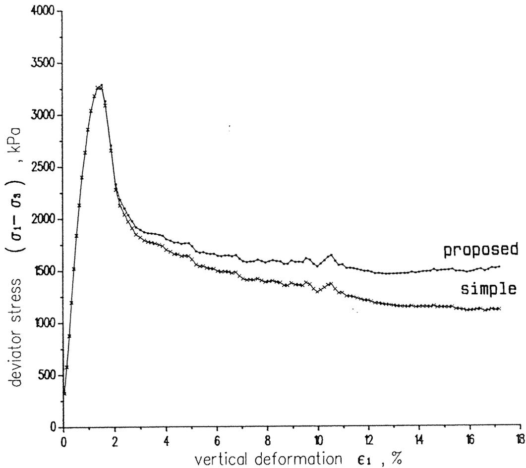
Fig. 8. Results of the CAD testing using silty clay with 10% cement, interpreted by the standard and the suggested method.
