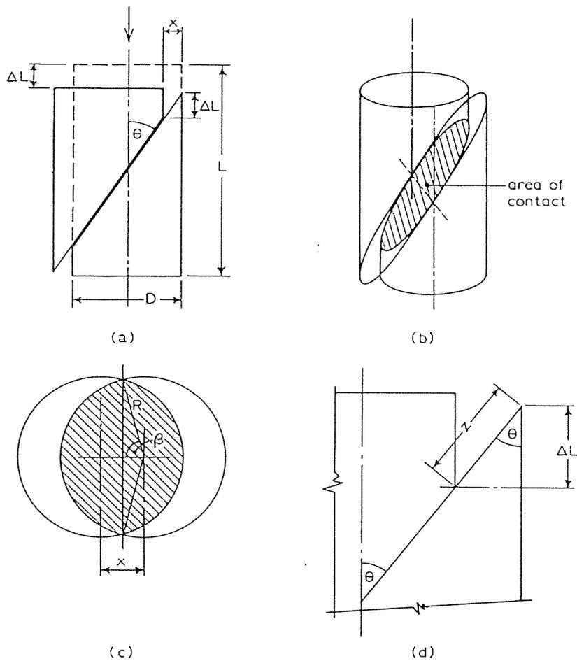
**Fig. 3. Area correction due to single-plane slip:**
