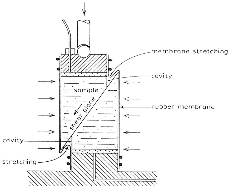
**Fig. 4. Rubber-membrane stretching due to single plane surface (after [4]).**
