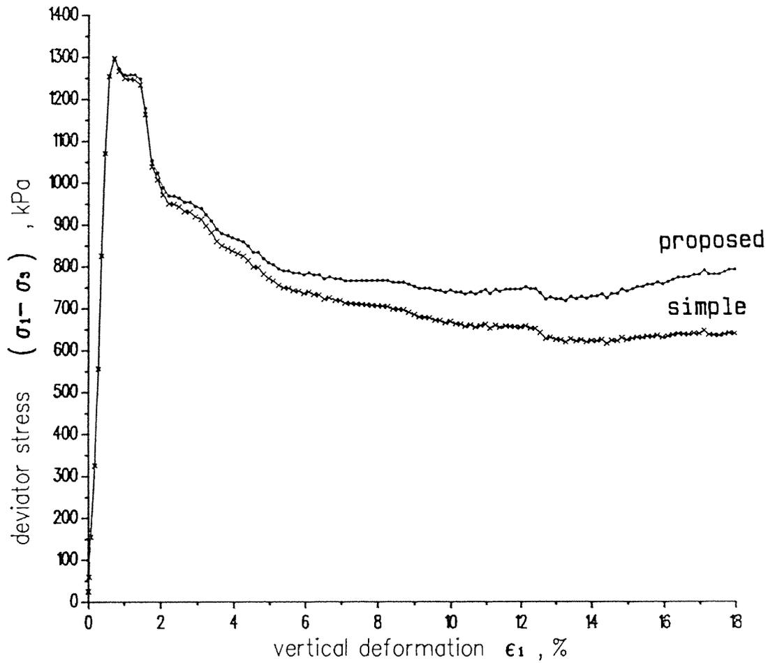
Fig. 9. CAU test results using silty clay with 10% lime+cement, interpreted by the "simple" and the suggested method.
